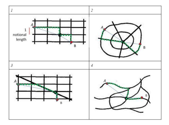
3. Calculate the length of the actual path (sum the length of all segments of the resulting path) and the aerial path (perform a similar action) in arbitrary units for all 4 diagrams. You can choose any artitrary unit of measurement. For example, the width of the street grid, as shown in Diagram 1. You may also use a scale of a helper measuring tool, such as a ruler.
