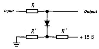
The selection of resistors for the reference voltage divider to calculate the voltage rating of the limiter is done using the formula:
