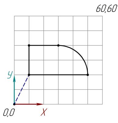
Indicate which of the G-CODE programs corresponds to it. Assume that the tool is initially located at point (0,0).
